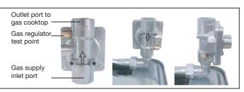
• ULPG connection: Using the supplied gas regulator, remove the dust seals on the inlet and outlet ports and position the outlet port of the regulator towards the gas inlet pipe of the cooktop. Using a suitable thread sealant, screw the regulator on and ensure that it is orientated with easy access to the test point. Connect the appropriate ULPG supply to the inlet port of the gas regulator.
