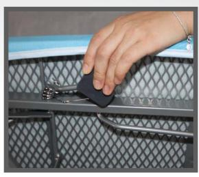
Adjusting Height: To increase or decrease the height of the ironing board, lift the release lever and either lift upwards or push downwards to reach the desired height setting. Release lever at desired height and wait for the click before releasing your grip on the board.
